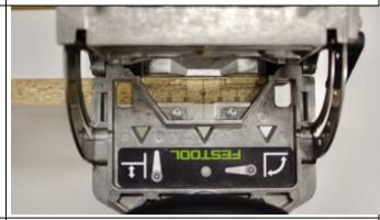
4 - Drilling female connector ACCURACY REQUIRED, NO TOLERANCE
