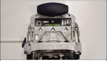
6 - Drilling tightening holes WITHOUT drill jig Use the marking hole on Festool Domino DF 500 Measure 15mm from edge.
